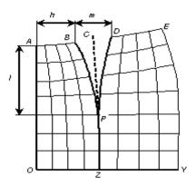
Figure 5 Position and sizes of contraction seams
