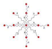
Figure 6 Springs and shock absorbers influencing a mass point.
